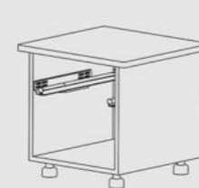
将左右滑动轨安装在柜子两侧) Assemble the left and right slide on both sides of cabinet
